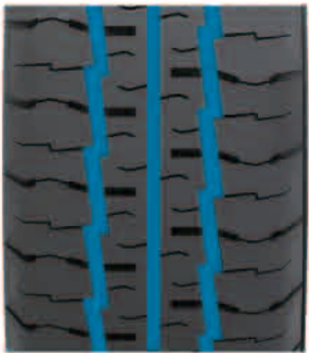
Three Longitudinal Grooves The three longitudinal grooves greatly enhance the drainage of tyres on wet land.
