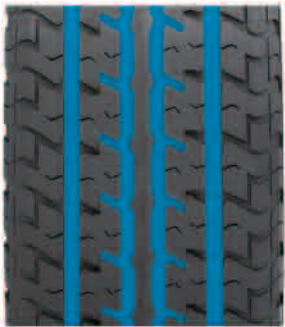
Drainage— four straight lines in the middle
