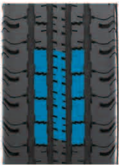
Grip — width variation design pattern groove.
