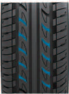
The six horizontal steps equally distributed can effectively decompose the pumping noise source, reduce noise, greatly promote the rigidity between the tread pattern blocks and eliminate sundries in the groove.
