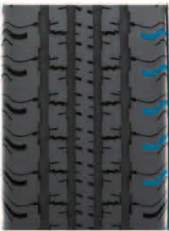
Wide and deep design on the shoulder offer more grip performance and heat release.
